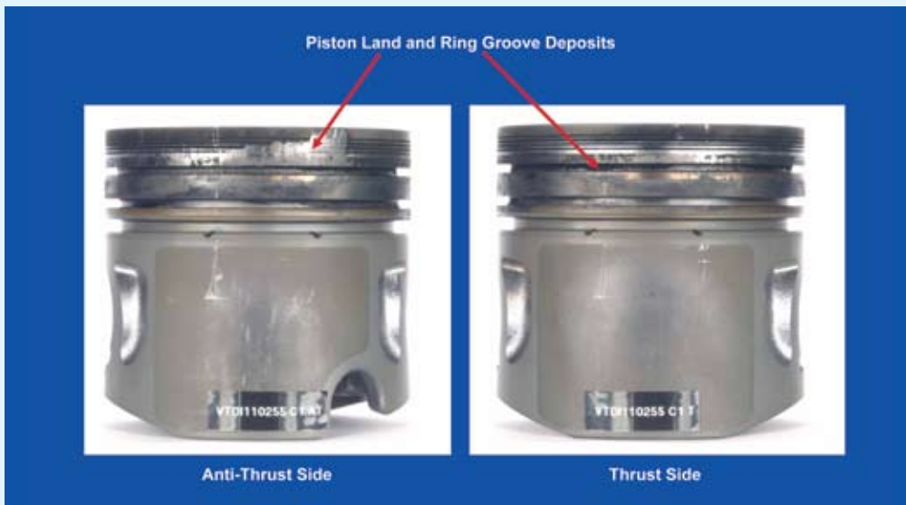
VW TDI Pistons After Test With Biodiesel
